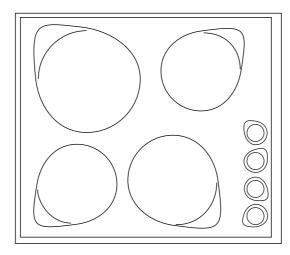
The hob is fitted with "Haloring" cooking zones with circular lamps and/or "Quickring" radiant cooking zones.
